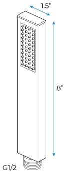
Flow Rate: 2.0 GPM / 7.6 LPM
